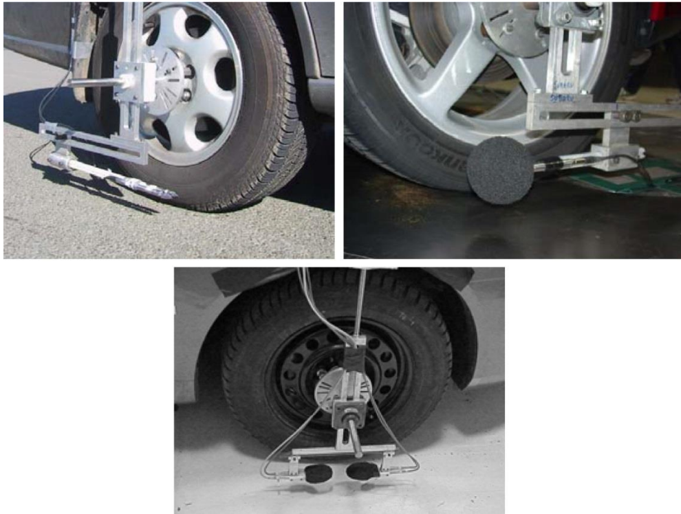
Figure 4-11: Photographs of wind noise reduction devices employed on different fixture configurations during wind tunnel testing, 2008
